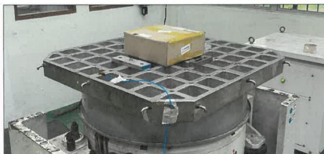
Figure 4: Loose load and vehicle vibration - Face 3 (base) facing down
