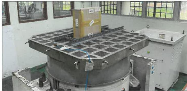
Figure 5: Loose load and vehicle vibration - Face 2 (side) facing down
