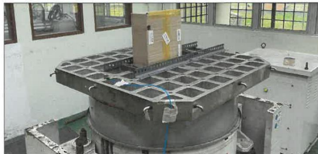
Figure 6: Loose load and vehicle vibration - Face 5 (end) facing down
